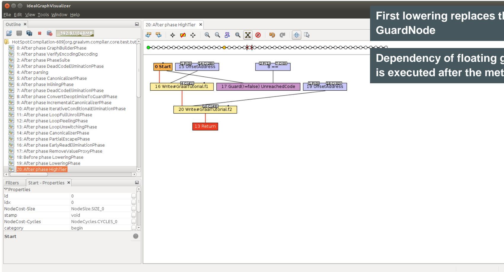
First lowering replaces the FixedGuardNode with a floating GuardNode
