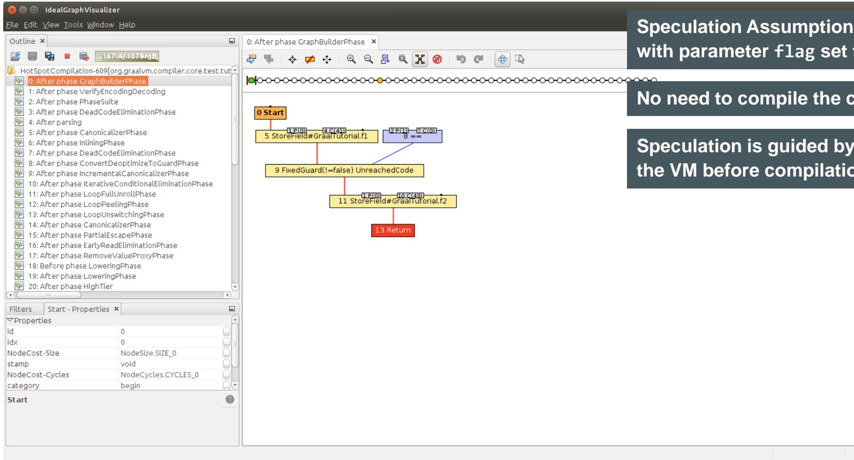
Speculation Assumption: method test is always called with parameter flag set to false
